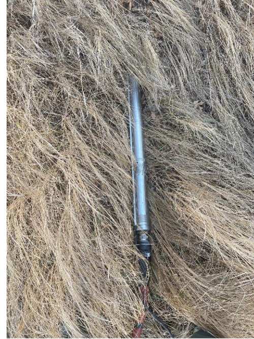
3-inch submersible pump for simultaneous purging
